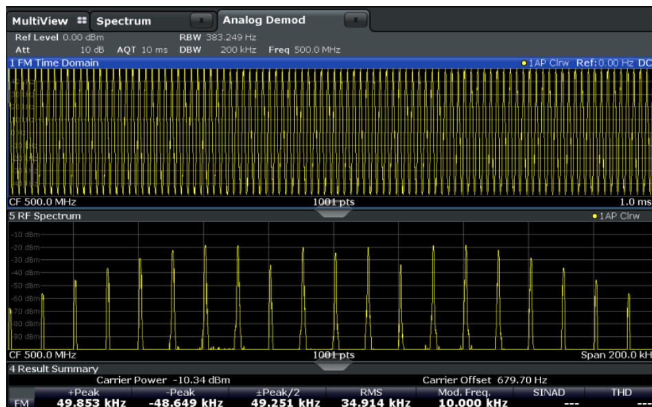
Fig. 9-5: RF spectrum with demodulation bandwidth = 200 kHz
