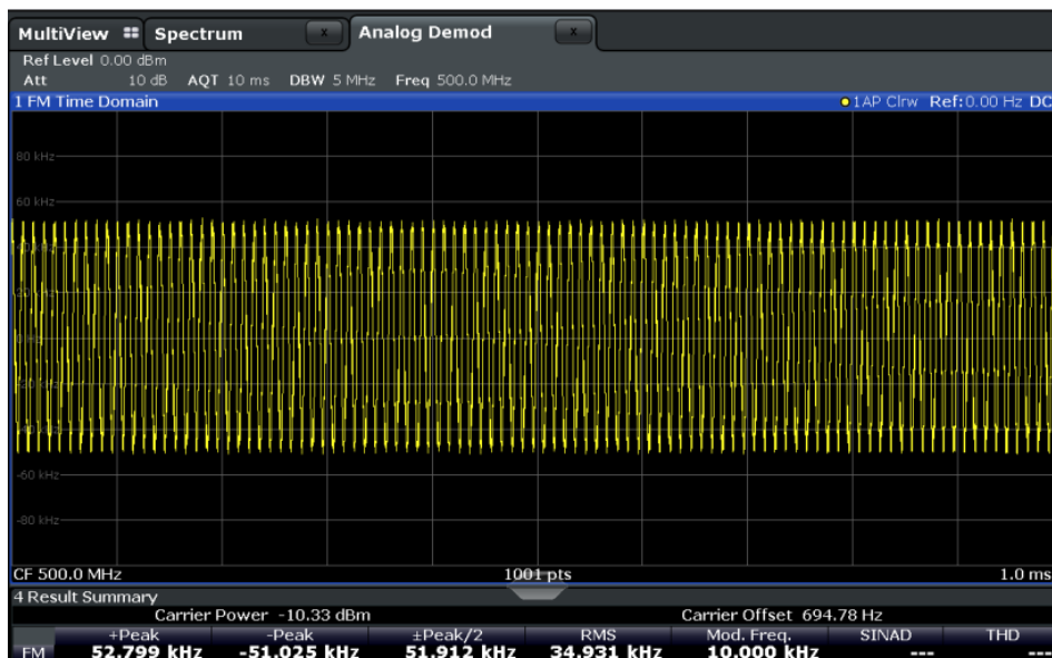
Fig. 9-3: Auto-scaled measurement of 10 signal periods (continuous)
